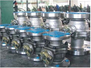
Size: 1/2" ~ 12" Class: 150 ~ 600 Floating Ball, Full & Reduced Bore Anti-Static Device Blow-out Proof Stem Fire Safe Design Optional Locking Device ISO 5211 Top Flange Back to content
