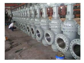
Size: 2" ~ 60"; Class: 150 ~ 1500; Slab or Expanding type Diversion hole type or non diversion hole
