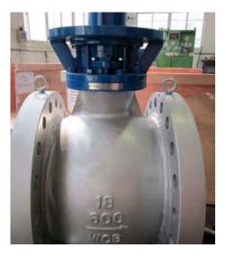
Size: 2" ~ 36" Class: 150 ~ 600 Metal to Metal Seat Trunnion Mounted Ball Leakage Rate Class IV ISO 5211Top Flange Back to content
