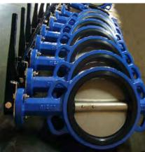
Size: 2" ~ 60" Class: 150 ~ 600 Wafer, Wafer-Lug or Double Flange Ends Concentric/ Double Eccentric Disc EPDM, NBR, PTFE, or VITON Seat Blow-out Proof Shaft Low Torque, Long Life Cycle ISO 5211Top Flange Back to content
